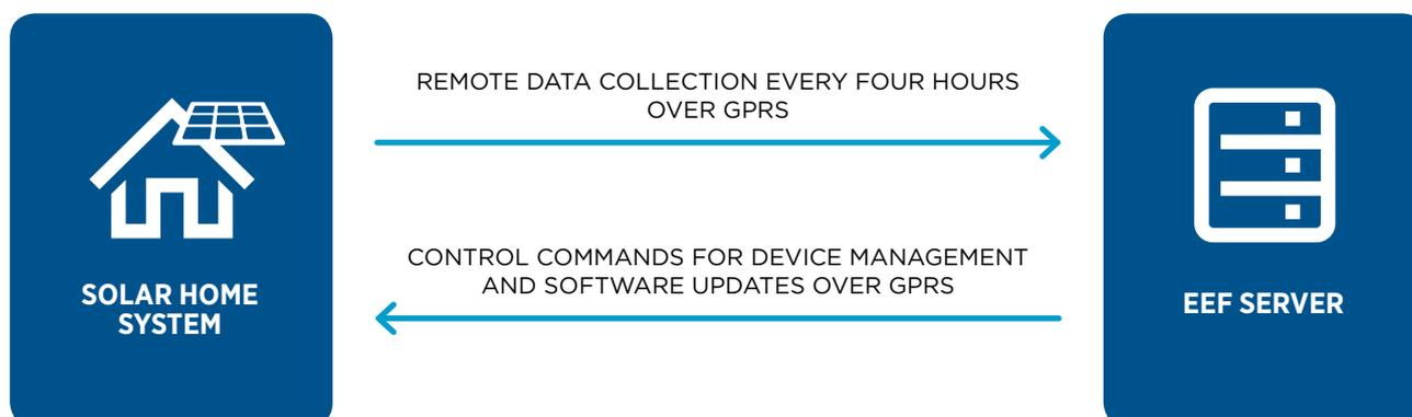
BBOX SHSs incorporate sensors and M2M communications to be able to control the SHS and monitor its health. They provide the ability to control the SHS with a variety of commands such as:
