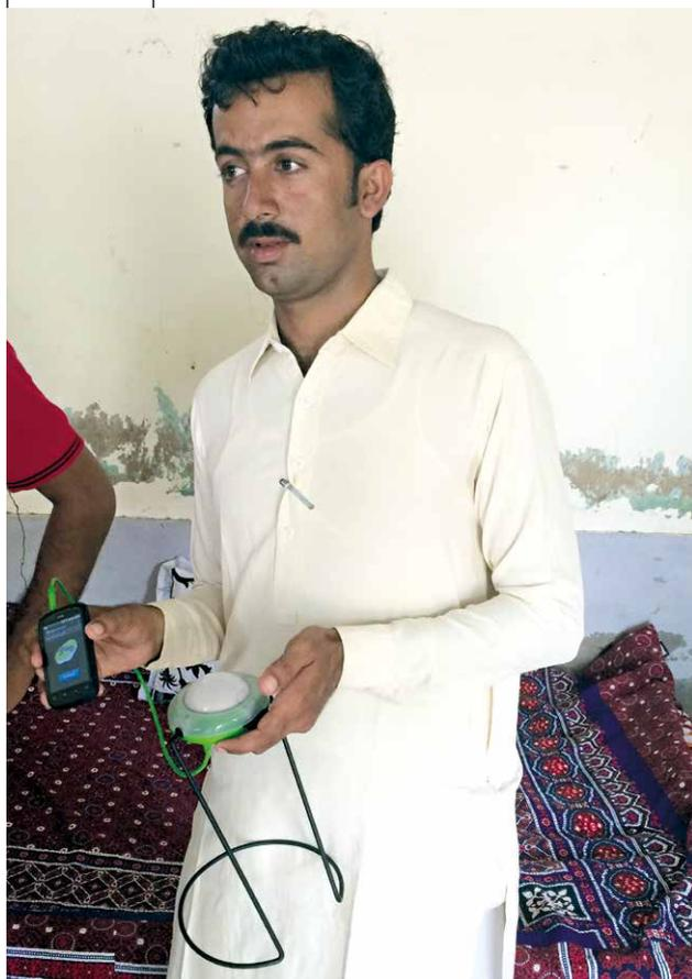
Lantern connected to smartphone for credit transfer
