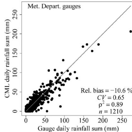
Each point on this scatterplot represents daily rainfall values for each location. The closest CML links are within 5 km of an official rain gauge, on average. The diagonal line represents perfect agreement between the measurements made by the rain gauges and from CML links, which would have a correlation coefficient of 1.
