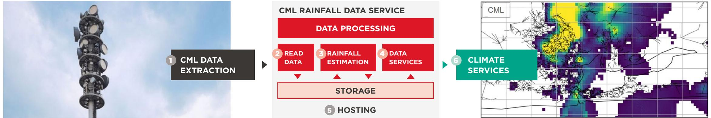
**1** CML data is acquired from mobile base stations through network management software, data loggers or dedicated software services. For example, the open source `pySNMPdaq` service has been developed to collect CML data directly from base stations, bypassing network management software.<sup>24</sup>
