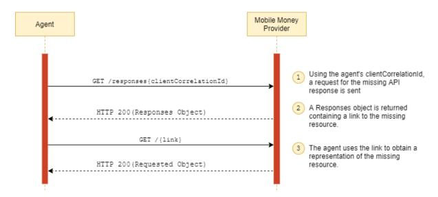
Figure 5-14 Retrieve a Missing API Response
