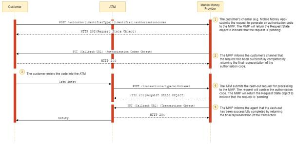
Figure 5-6 Customer Withdrawal at an ATM using a Pre-authorised Cash-out Code
