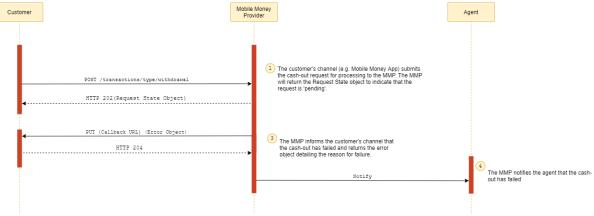
Figure 5-5 Customer-initiated Cash-out Failure
