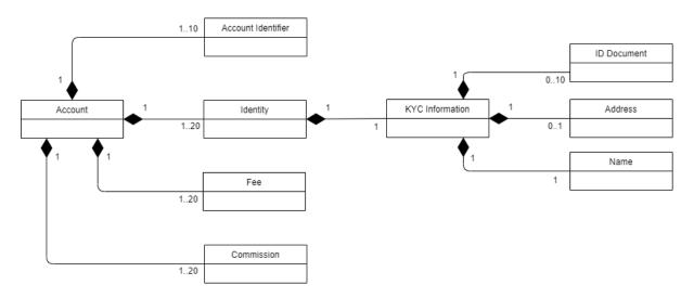
Figure 2-3 Account Creation UML Class Diagram
