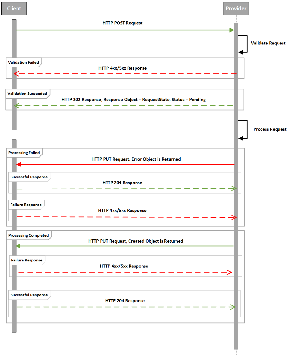
Figure 3: Mobile Money API Asynchronous Callback Diagram for Create Requests
