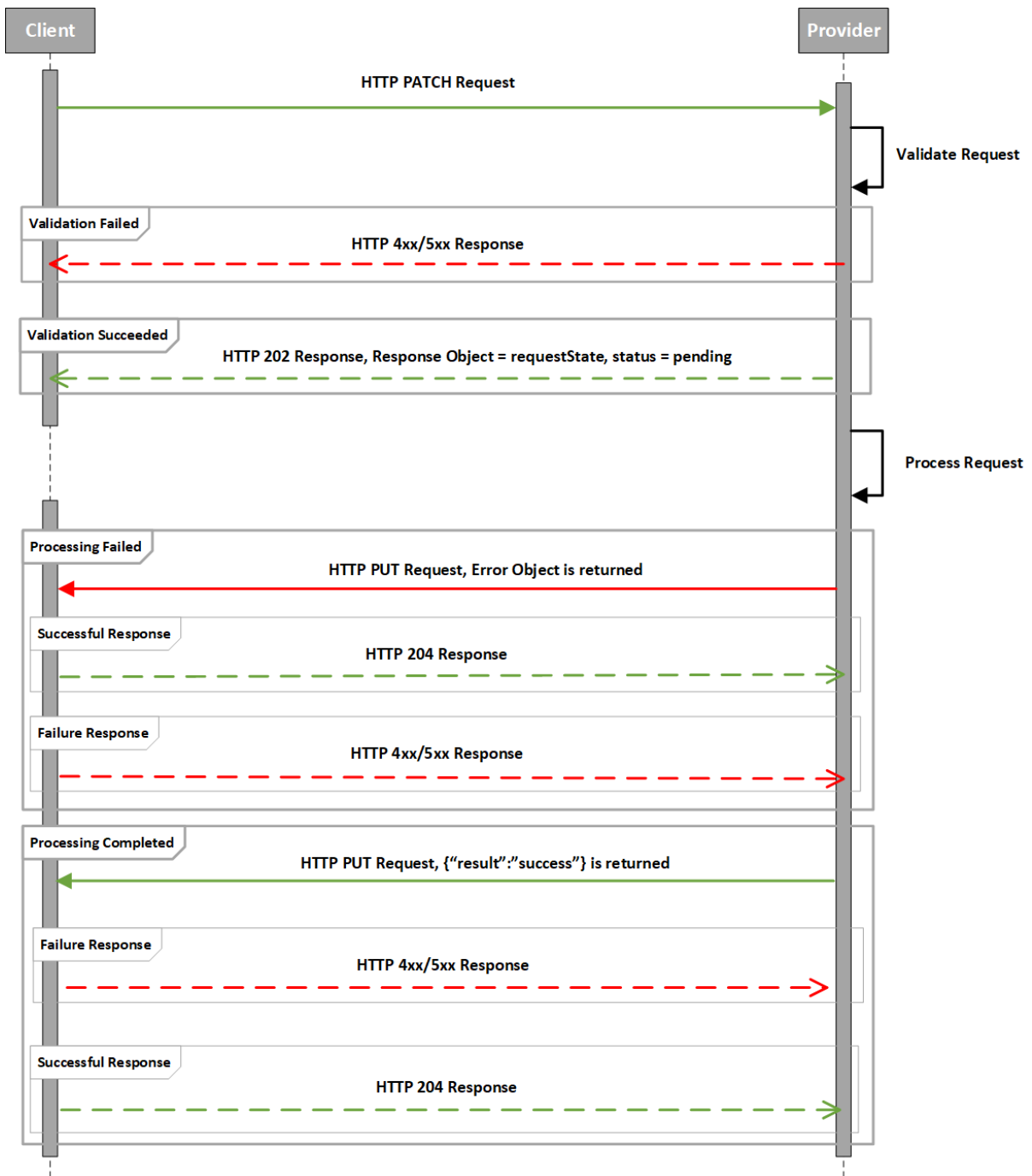
Figure 6: Mobile Money API Asynchronous Callback Diagram for Update Requests
