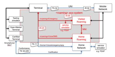
Figure 2: VoLTE Test Ecosystem
