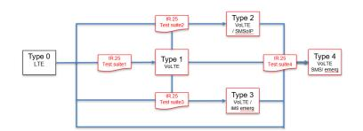
Figure 3: VoLTE evolving types & test suites applied
