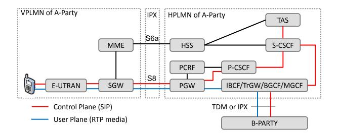
Figure 1: S8HR VoLTE Roaming Architecture
