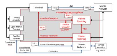
Figure 2: VoLTE Test Ecosystem
