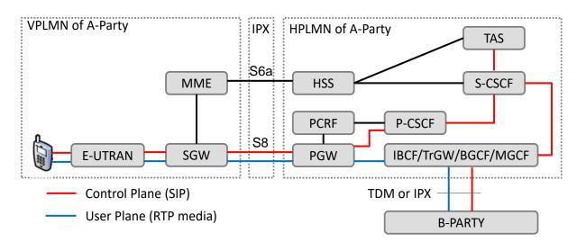
Figure 1: S8HR VoLTE Roaming Architecture
