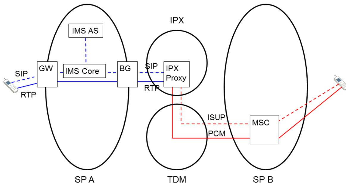
**Figure A-4: IMS-to-MSC Voice NNI with IPX performing the TDM breakout**
