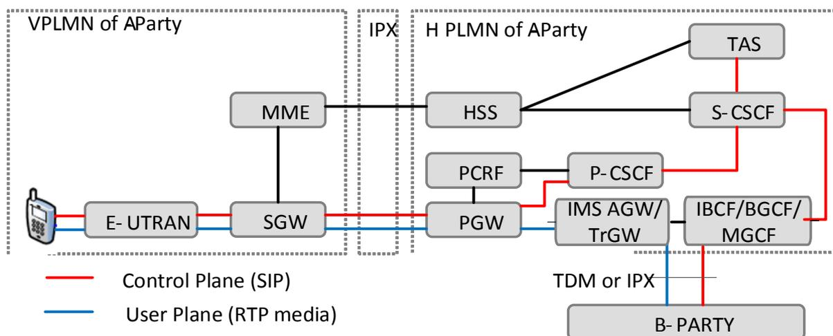
**Figure 2-8: S8HR IMS Roaming Architecture (VoIMS service shown)**
