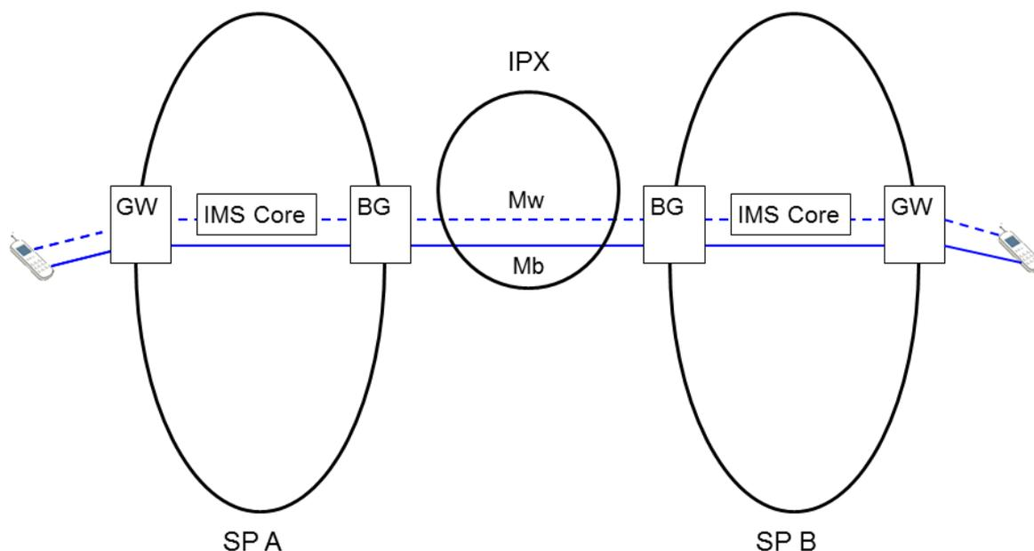
**Figure 3-3: IMS interconnection using Mw & Mb Interfaces (simplified example not showing e.g. FW nodes)**
