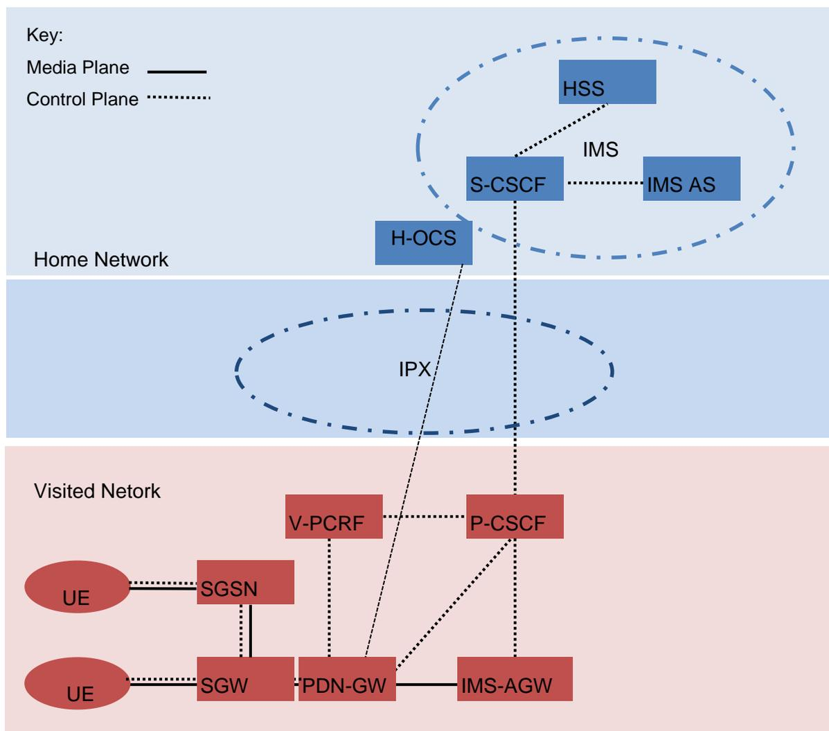
**Figure 2-6: Voice Roaming Architecture using LBO – EPC**
