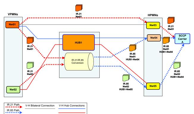
In case where relation (roaming or interworking) will be established through only one HUB, the process drawn in the above picture must be used. The process will be the same in case of Client Operators and Connected Operators.
