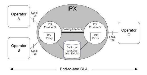
Figure 1: High-Level View of IPX (from IR.34)
