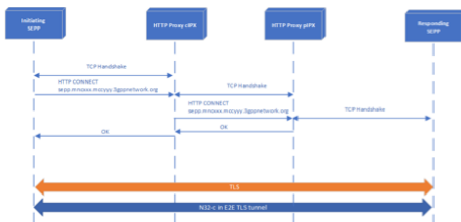
Figure 50 - N32-c mTLS connection using HTTP CONNECT
