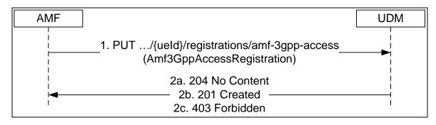
Figure 10 AMF Registering for 3GPP access [10] Section 5.3.2.2.2
