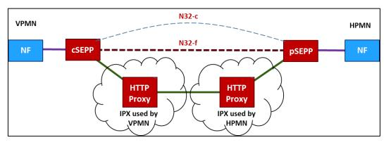
Figure 7 End to end HTTP/2 Roaming Architecture
