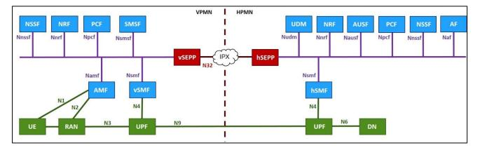
Figure 3 5G System Roaming architecture – Service Based Interface Representation (HR)
