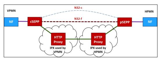
Figure 8 - End to end HTTP/2 Roaming Architecture
