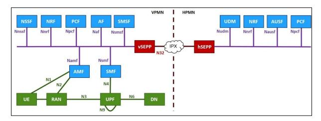
Figure 1 – 5G System Roaming architecture – Service Based Interface Representation (LBO)
