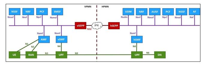
Figure 4 – 5G System Roaming architecture – Service Based Interface Representation (HR)
