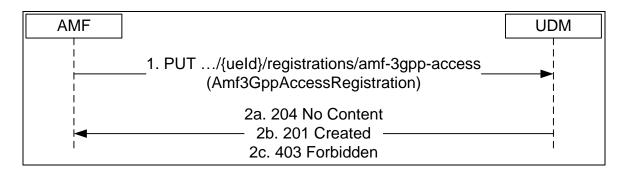
Figure 13 – AMF Registering for 3GPP access [10] Section 5.3.2.2.2
