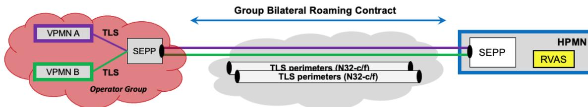
**Figure 25 Bilateral scenario between Mobile Operator Groups with a shared Group SEPP**
