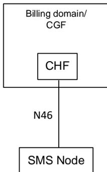
**Figure 20– 5G Reference point Representation (sms charging)**
