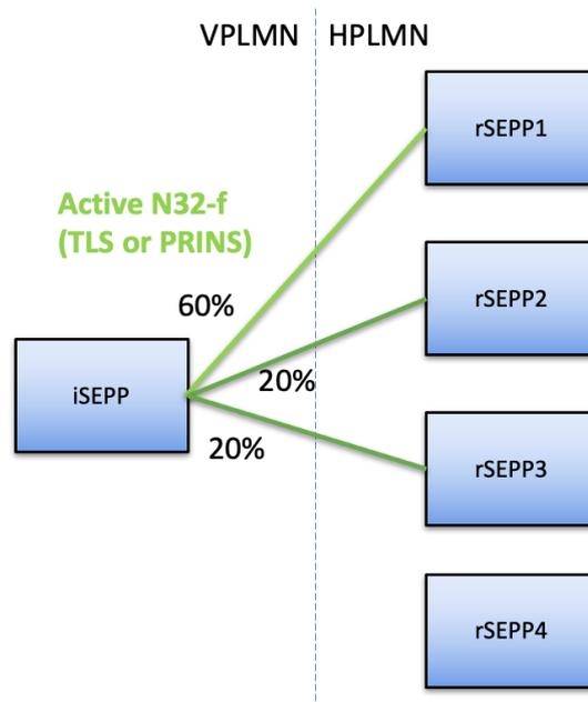
**Figure 9 – Sample load distribution over rSEPPs**
