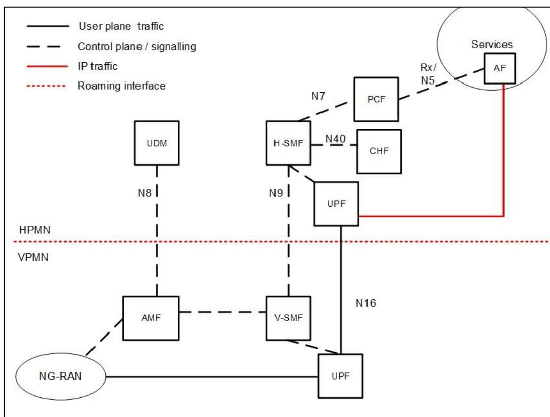
**Figure 22 – PCC Architecture with Home Routed Architecture**
