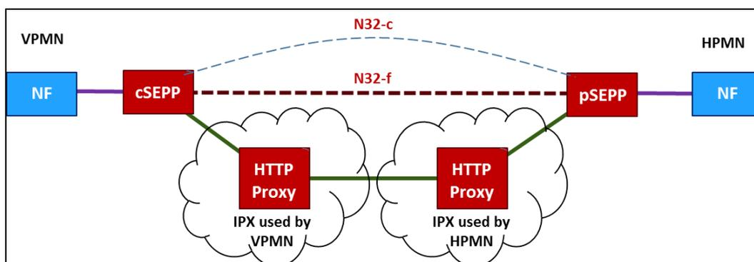
**Figure 8 – End to end HTTP/2 Roaming Architecture**
