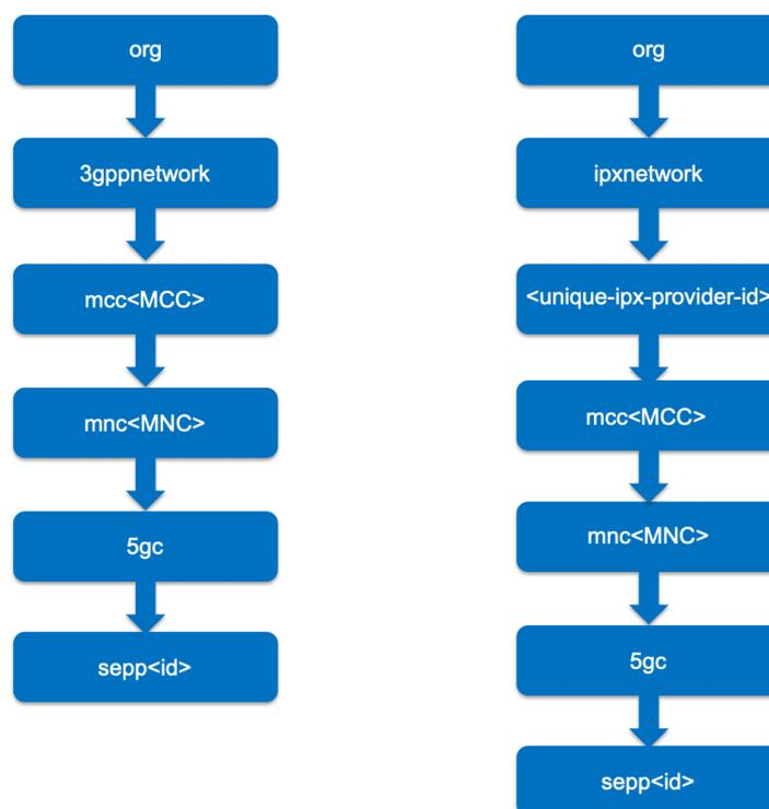
**Figure 10– FQDN hierarchy for MNO (left) and FQDN hierarchy for non-MNO (right)**
