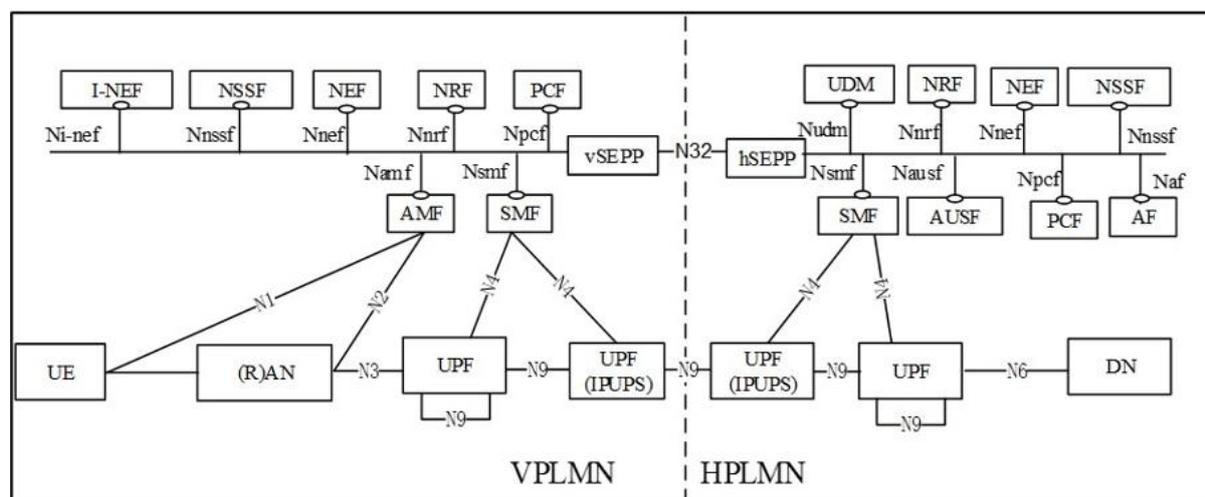
**Figure 14 Roaming Home Routing Scenario – In Served Based Interface Presentation**
