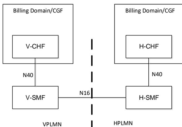
**Figure 17– 5G Reference point Representation (data HR charging)**
