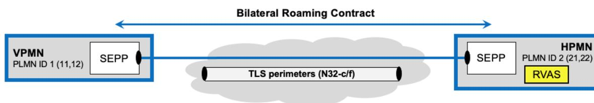
Figure 23 Bilateral scenario between VPMN and HPMN with internal SEPPs
