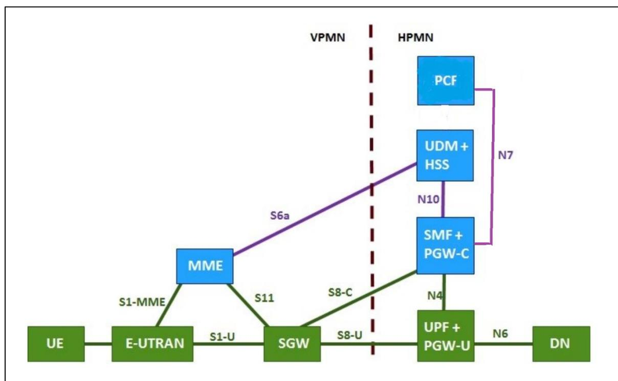
**Figure 11 – Home-routed roaming architecture for interworking between 5GS EPC/E-UTRAN**
