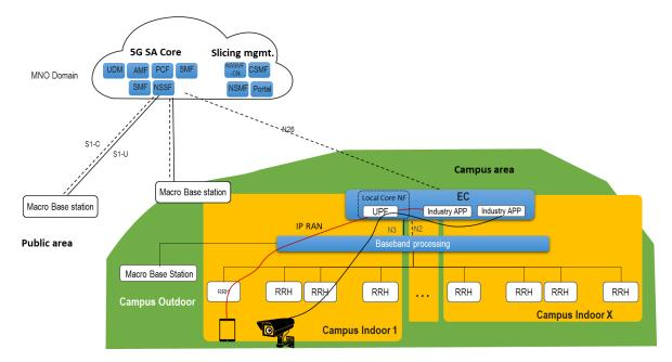
Figure 3: NPN deployment example case
