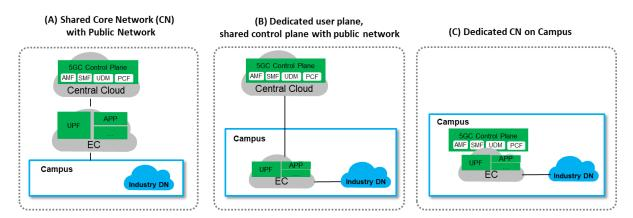
Figure 2: NPN deployment - Core Network Options
