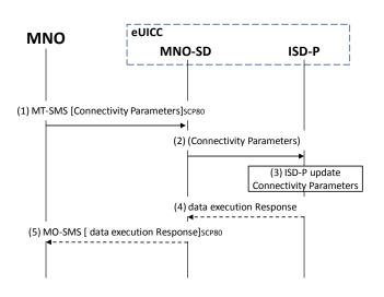
Figure 28: Connectivity Parameters Update by MNO
