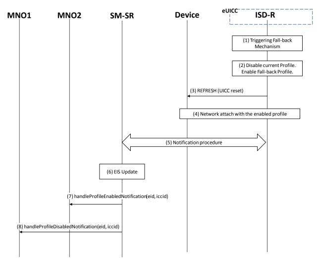
Figure 32: Fall-Back Activation Procedure
