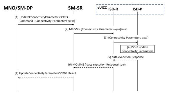
Figure 29: Connectivity Parameters Update Using SCP03
