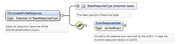
Figure 102: <rps:ES3-EnableProfileResponse>
