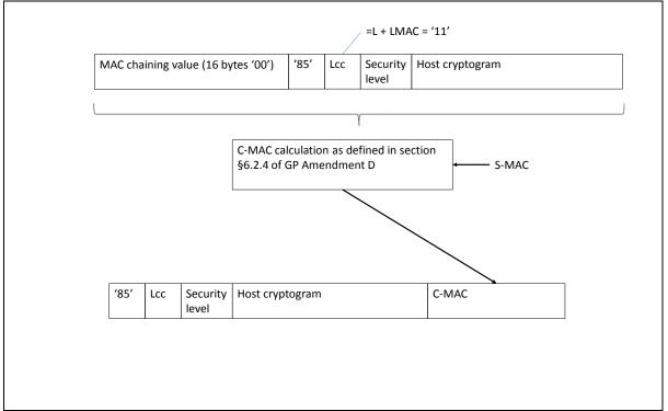
Figure 33: TLV Command Data Field Encryption
