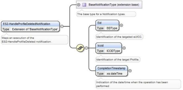
Figure 86: <rps:ES2-HandleProfileDeletedNotification >
