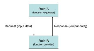
Figure 36: Functions as a Request-Response Data Exchange
