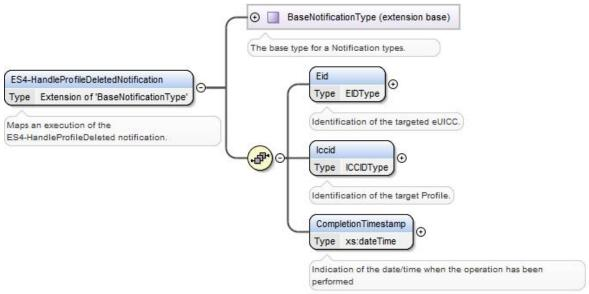
Figure 134: <rps:ES4-HandleProfileDeletedNotification>
