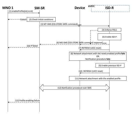
Figure 16: Profile Enabling failure, with roll-back
