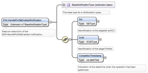
Figure 132: <rps:ES4-HandleProfileEnabledNotification>
