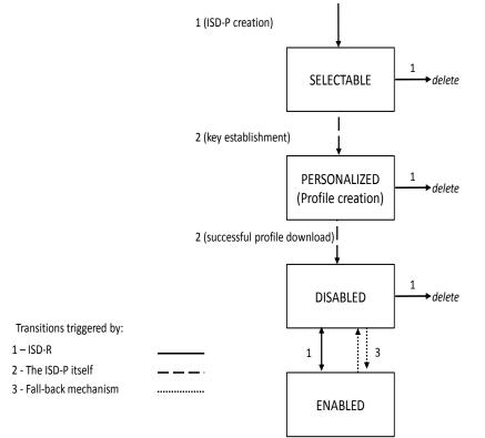
Figure 3: ISD-P Life-Cycle State Transitions
