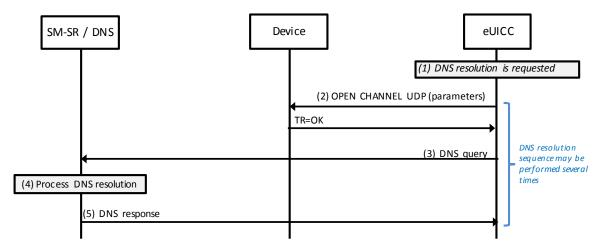
Figure 10: Sequence for Basic DNS resolution
