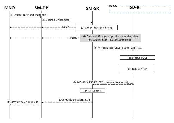
Figure 22: Profile and ISD-P Deletion via SM-DP
