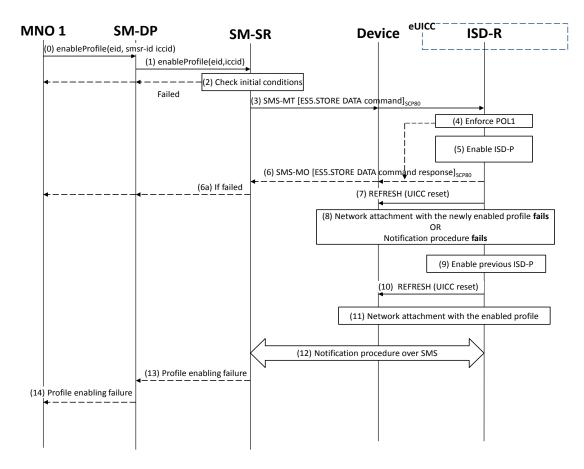
Figure 18: Profile Enabling, With Roll-Back
