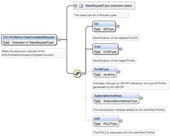
Figure 95: <rps:ES3-ProfileDownloadCompleted Request>
