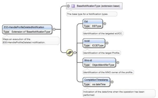
Figure 112: <rps:ES3-HandleProfileDeletedNotification>
