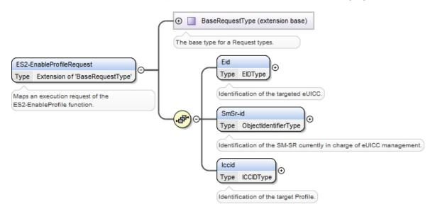
Figure 77: <rps:ES2-EnableProfile Request>
