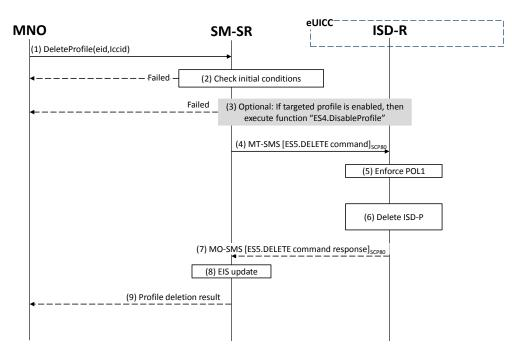
Figure 21: Profile and ISD-P Deletion
