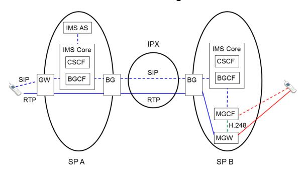
Figure A-1: IMS-to-IMS Voice NNI with receiver using CS UNI
