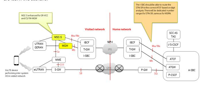
Figure 2-9 - SRVCC with SIP-I Architecture
