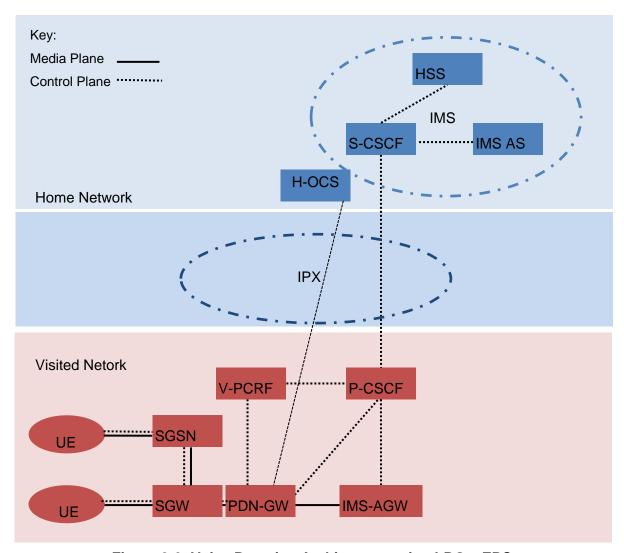
Figure 2-6: Voice Roaming Architecture using LBO - EPC
