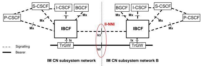
Figure 3-2: IMS interconnection using Ici & Izi Interfaces (from 3GPP TS 23.228)
