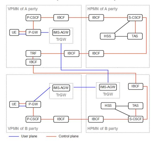
Figure 2-4: Control and User Plane Routing – LBO-VR
