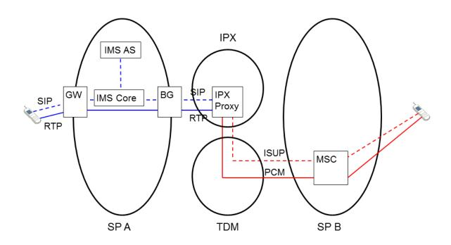
Figure A-4: IMS-to-MSC Voice NNI with IPX performing the TDM breakout
