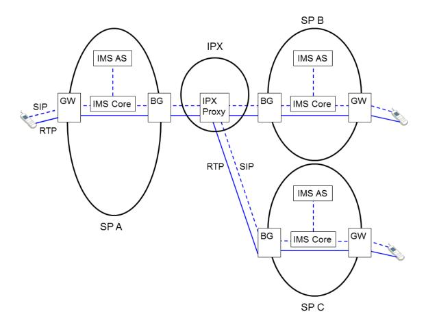
Figure 5-4: VolMS NNI (Hubbing Model)
