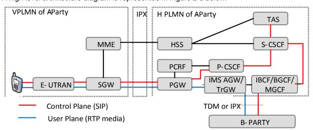
Figure 2-8: S8HR IMS Roaming Architecture (VoIMS service shown)
