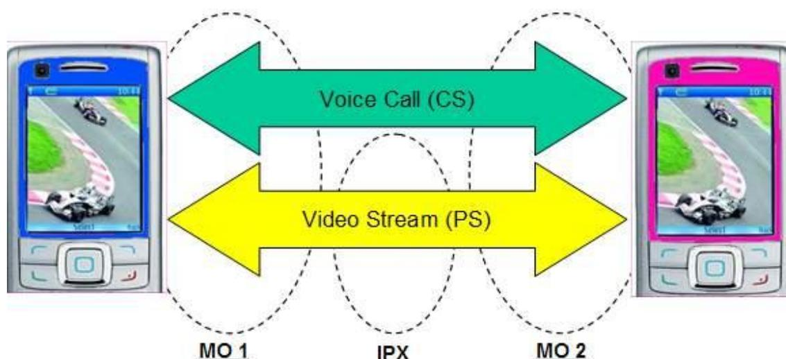
**Figure 1 High-Level Figure of Video Share Connection**
