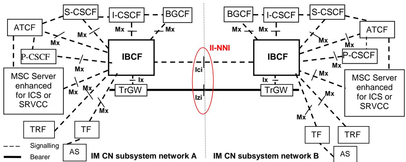
**Figure 1 : Inter IMS NNI Reference Architecture**
