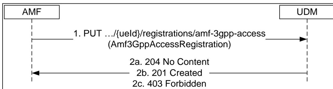
**Figure 10 AMF Registering for 3GPP access [10] Section 5.3.2.2.2**
