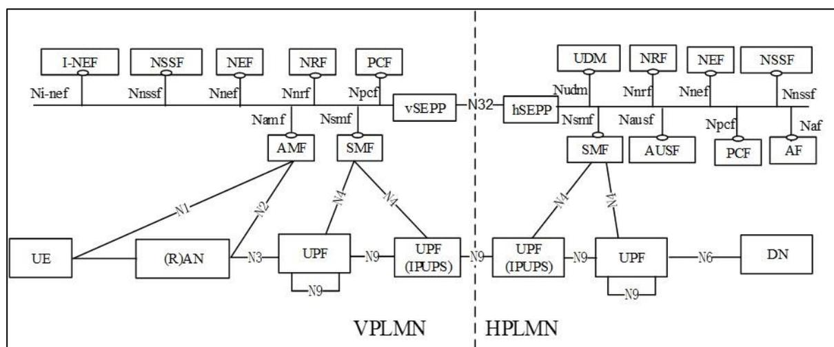
**Figure 11 Roaming Home Routing Scenario – In Serviced Based Interface Presentation**
