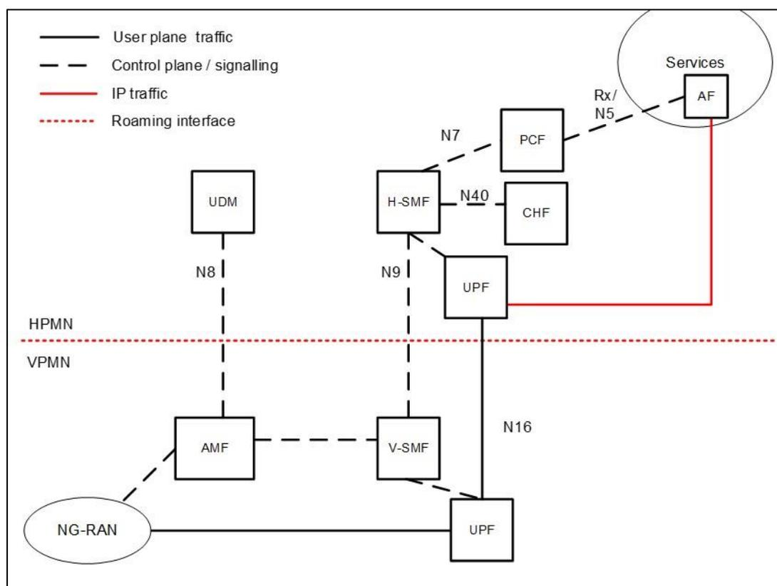
**Figure 14 PCC Architecture with Home Routed Architecture**
