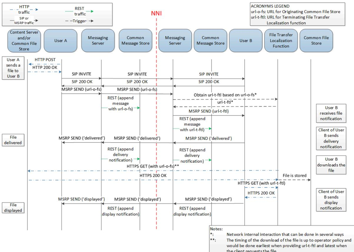
Figure 15: File Transfer Localisation Function: global flow
