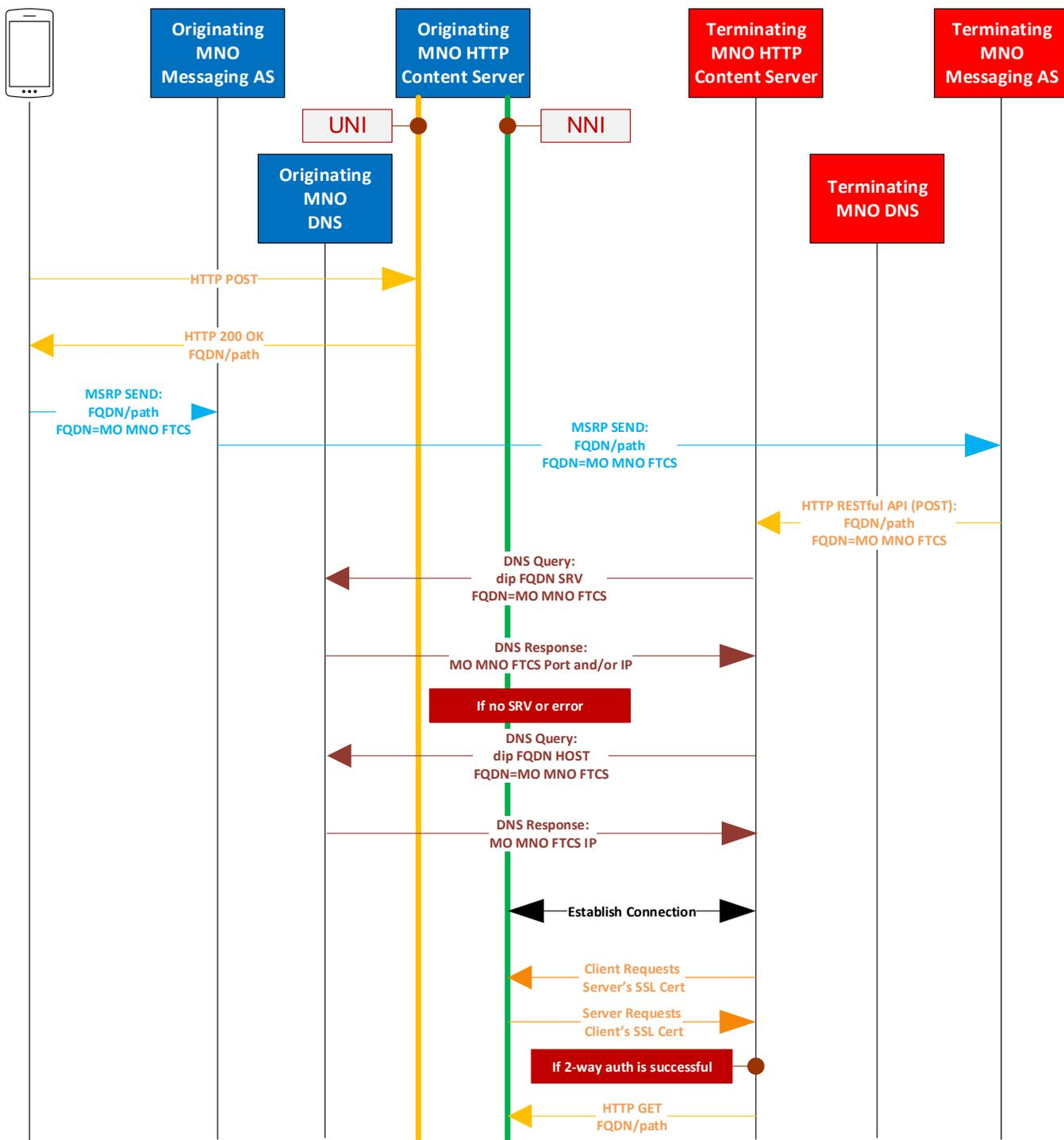
**Figure 16: Mutual Authentication for HTTP File Transfer Localization Option 1 (SRV based)**
