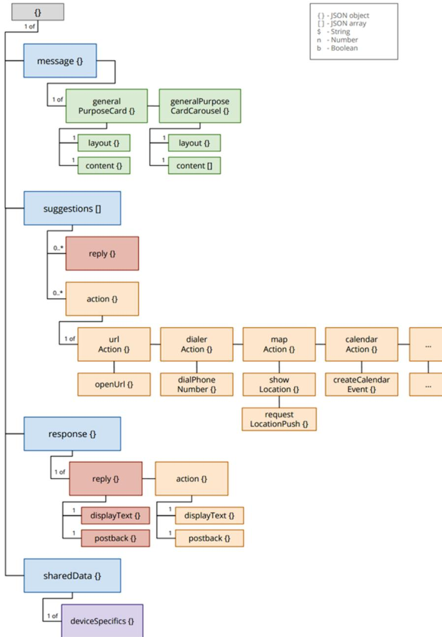
Figure 10: JSON message payloads data structure overview
