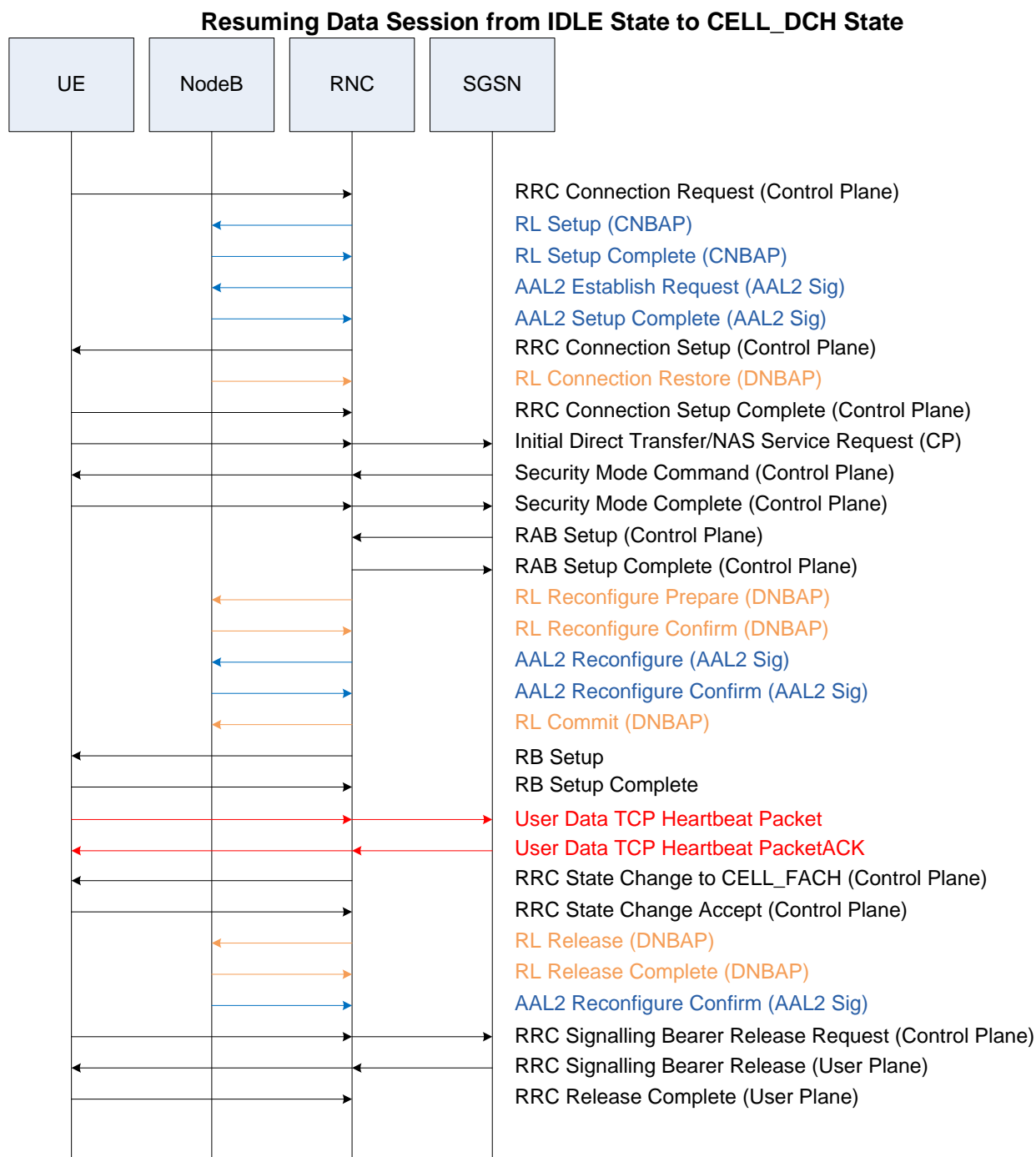
Figure 10 - Idle State to CELL_DCH State
