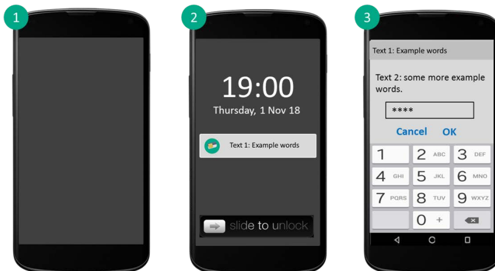
Figure 6: GET INPUT STK proactive command arriving on a device in locked screen
