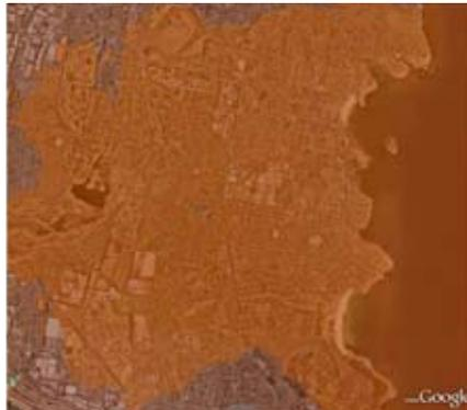
**Figure 8.** The orange areas are predictions of the places where indoor mobile service coverage is maintained should power reductions be imposed to meet a 3 V/m limit.
