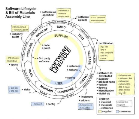
Figure 1: The Software lifecycle with multiple stages where underlying code might change, and thus the SBOM would be updated to reflect the changes.
