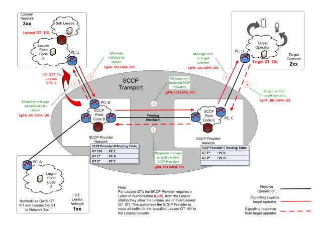
Figure 4 - Routing via Lessee Only Signalling Flow
