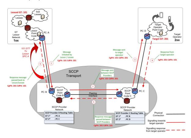
Figure 3 - Routing via Lessor Signalling Flow
