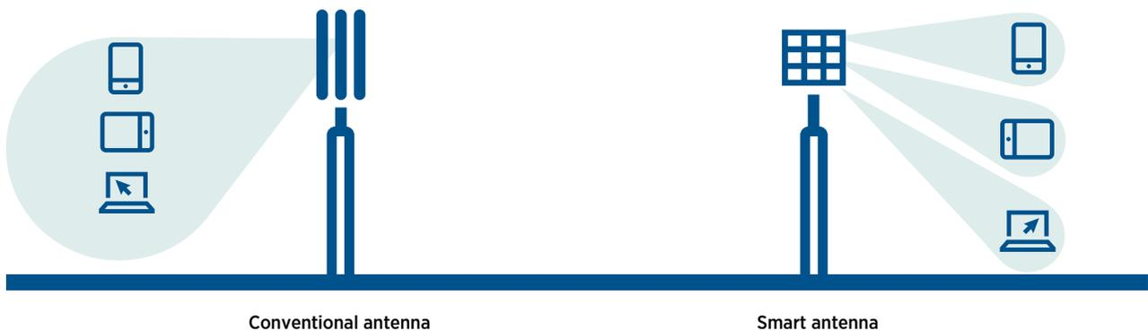
As shown in Figure 10, a conventional base station antenna transmits a radio signal to a wide area regardless of how many users are connected. Smart beam forming antennas transmit radio signals only to connected users reducing interference and exposure. Beamforming involves combining the signal from multiple antennas to improve performance. However, operation at higher frequencies means that the size of
