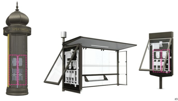
Figure 37 – Illustration of small cells integration in street furniture
