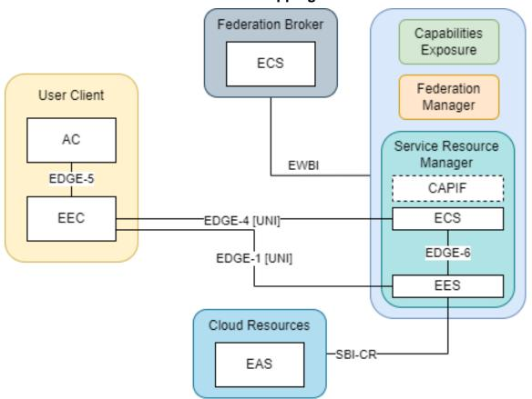
Figure 5: EDGEAPP Functional element mapping to Operator Platform
