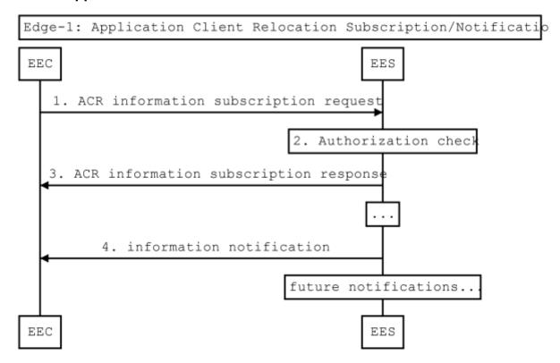
Figure 9: Application Client Relocation (from 3GPP TS 23.558 [6])
