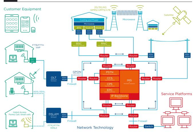
RAN equipment: RRU/BBU; 2G BTS; 3G node B/RNC; 4G eNodeB; 5G antenna; Massive MIMO
