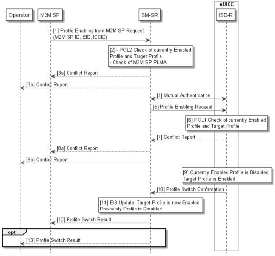
Figure 18: Profile Enabling via M2M SP
