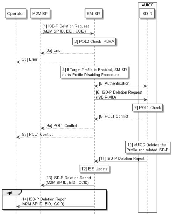
Figure 20: ISD-P Deletion via M2M SP
