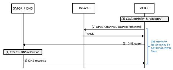
Figure 10: Sequence for Basic DNS resolution
