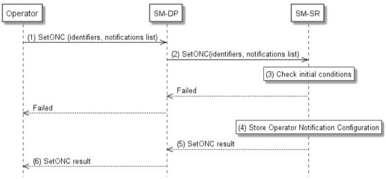
Figure 42: Set Operator Notification Configuration via SM-DP
