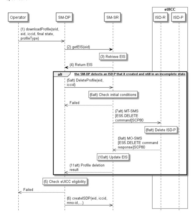
Figure 315-A: ISD-P cleanup at the beginning of a subsequent profile download
