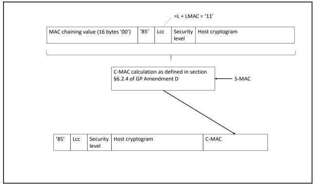
Figure 45: C-MAC Computation for External Authenticate Command TLV
