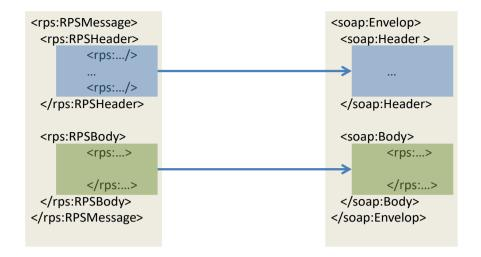
Figure 141: RPS Message Binding
