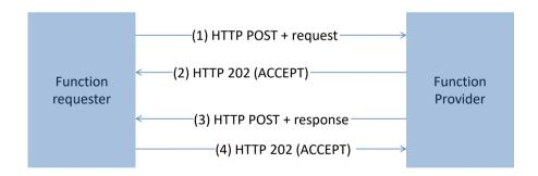
Figure 143: MEP: Asynchronous Request-Response With Callback
