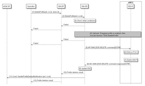
Figure 22: Profile and ISD-P Deletion via SM-DP
