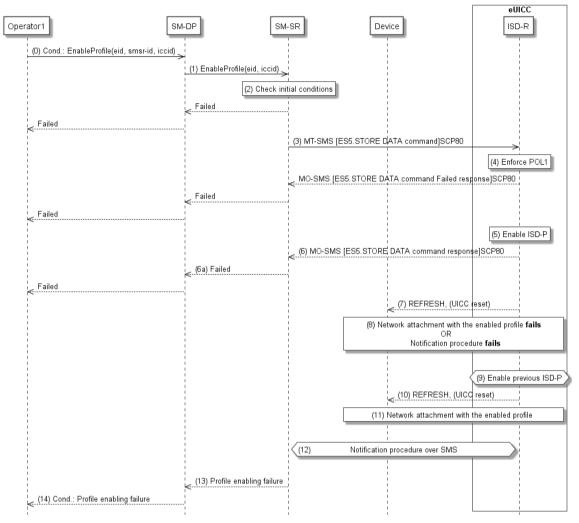
Figure 18: Profile Enabling, With Roll-Back
