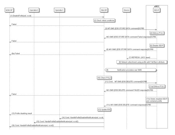
Figure 35: Profile Disabling via M2M SP
