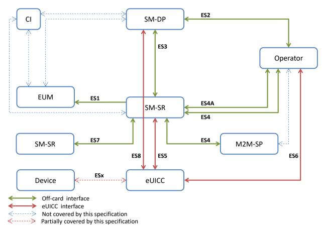
Figure 1: eUICC Remote Provisioning System
