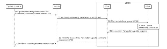
Figure 29: Connectivity Parameters Update Using SCP03
