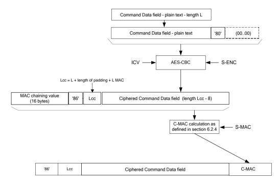
Figure 46: TLV Command Data Field Encryption
