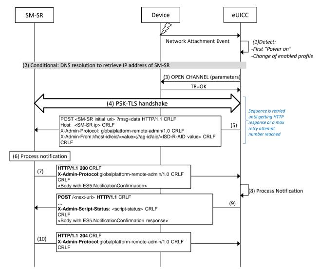
Figure 31: Sequence Flow of Notification Over HTTPS
