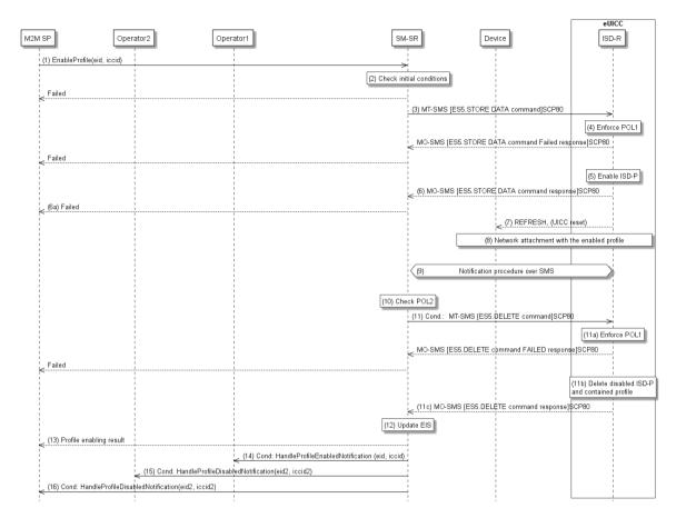
Figure 33: Profile Enabling via M2M SP, Success Case
