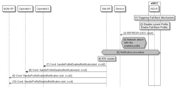
Figure 32: Fall-Back Activation Procedure
