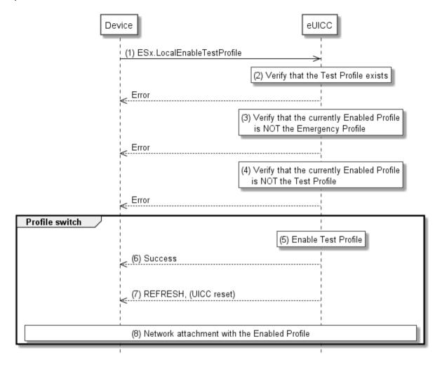
Figure 322: Local Enable of Test Profile
