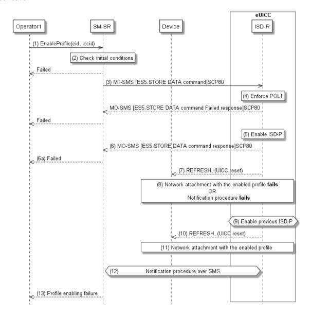
Figure 16: Profile Enabling failure, with roll-back
