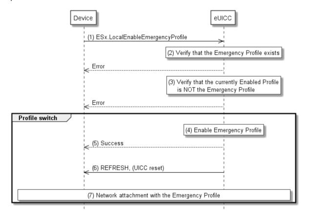
Figure 330: Local Enable of Emergency Profile
