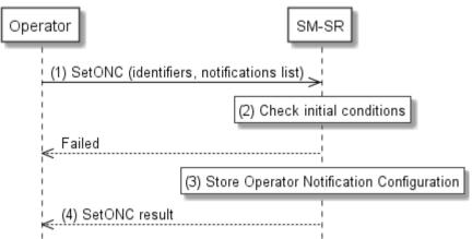
Figure 3211-A: Set Operator Notification Configuration
