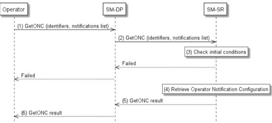
Figure 44: Retrieve Operator Notification Configuration via SM-DP
