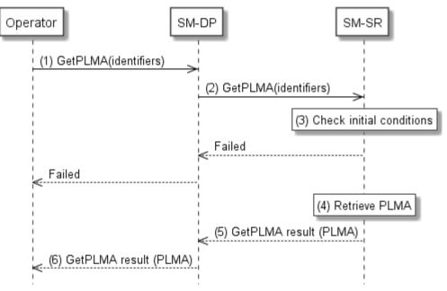
Figure 40: Retrieve PLM A by Operator via SM-DP
