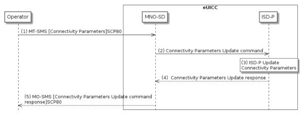
Figure 28: Connectivity Parameters Update by Operator
