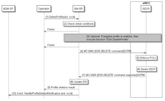
Figure 21: Profile and ISD-P Deletion
