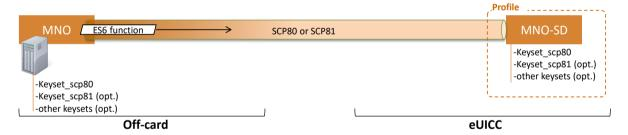
Figure 7: Secure Channel Between Operator and MNO-SD
