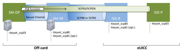
Figure 6: Secure Channel Between SM-DP and ISD-P
