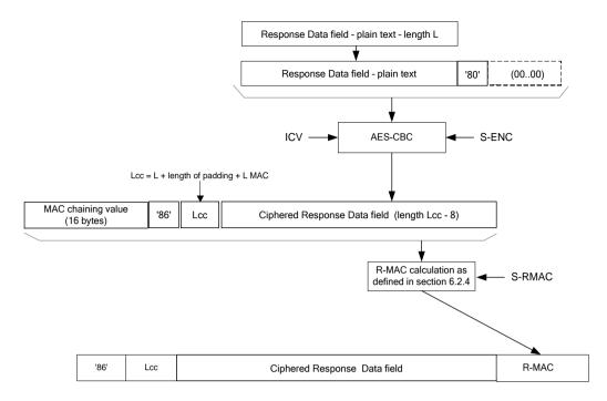
Figure 47: TLV Response Data Field Encryption
