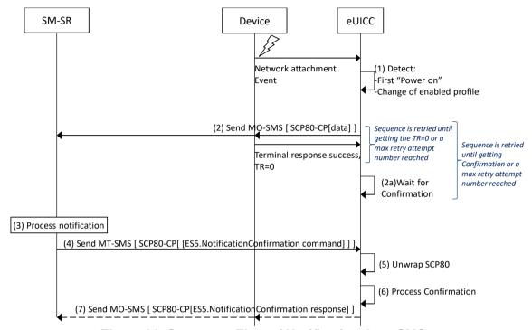
Figure 30: Sequence Flow of Notification Over SMS
