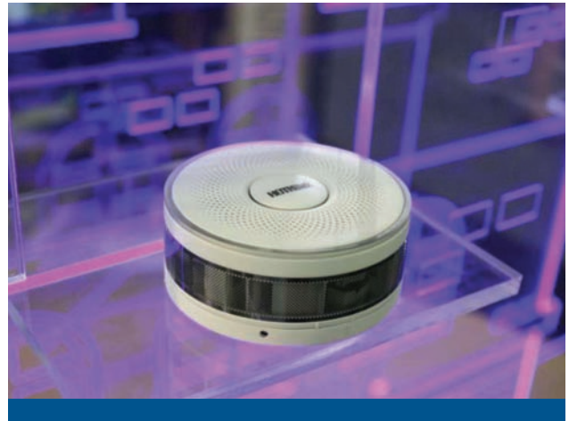
Figure 11: A Hothink detector connected via NB-IoT
