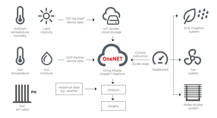
**Figure 6** The OneNET Platform aggregates data from OCP partner devices and from "off the shelf" device vendor cloud services and manages access to the stored data by integrated smart hardware solutions (such as irrigation) and analytic applications.
