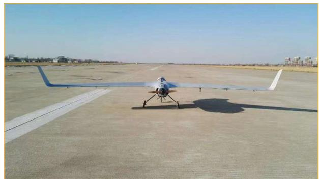
**Figure 1** Hybrid wing high-altitude long-endurance UAV
