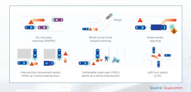
**Protecting vulnerable road users:** Vehicles equipped with C-V2X systems will in future be able to detect the smartphones of pedestrians and cyclists, enabling them to avoid collisions with these vulnerable road users. When a smartphone detects it is on or near a road, it could use C-V2X to continually broadcast a signal to warn nearby connected vehicles of its presence.
