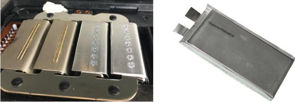
2KW Fibre laser with depth monitoring of welds
