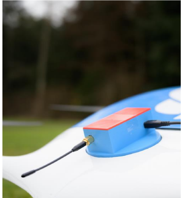
Figure 7: Swisscom Cellular Network Remote ID Device
