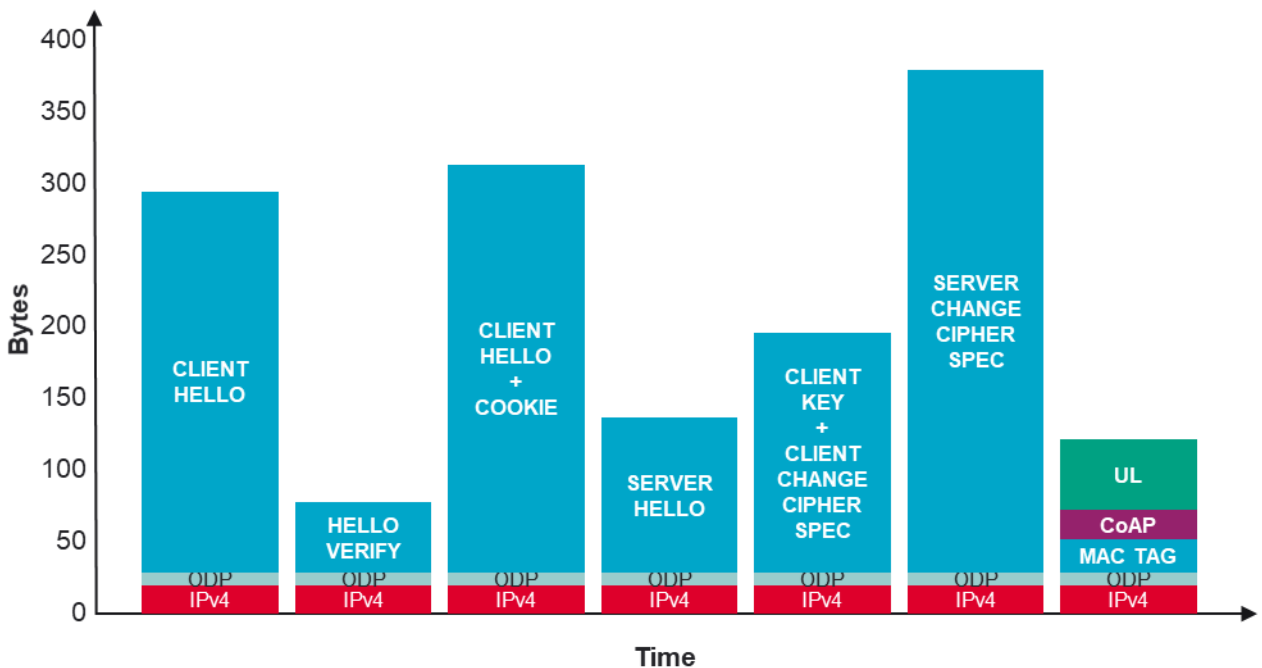
Figure 5 – CoAP with DTLS – using TLS_PSK_WITH_AES_256_CBC_SHA384
