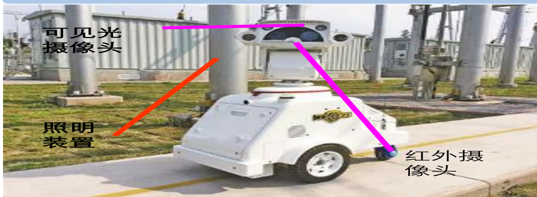
Inspection robot : 2~4 HD video + various sensors
