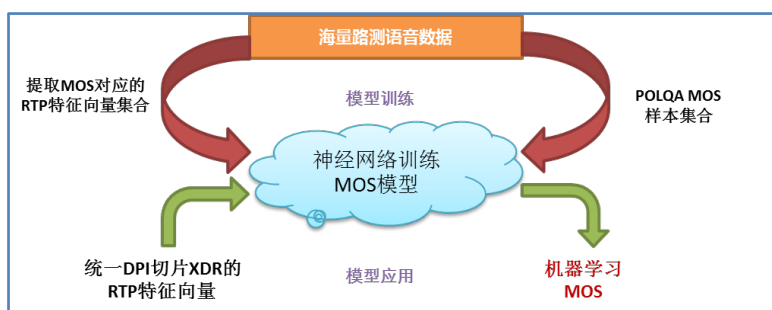
Figure 51: MOS model training by using a neural network
