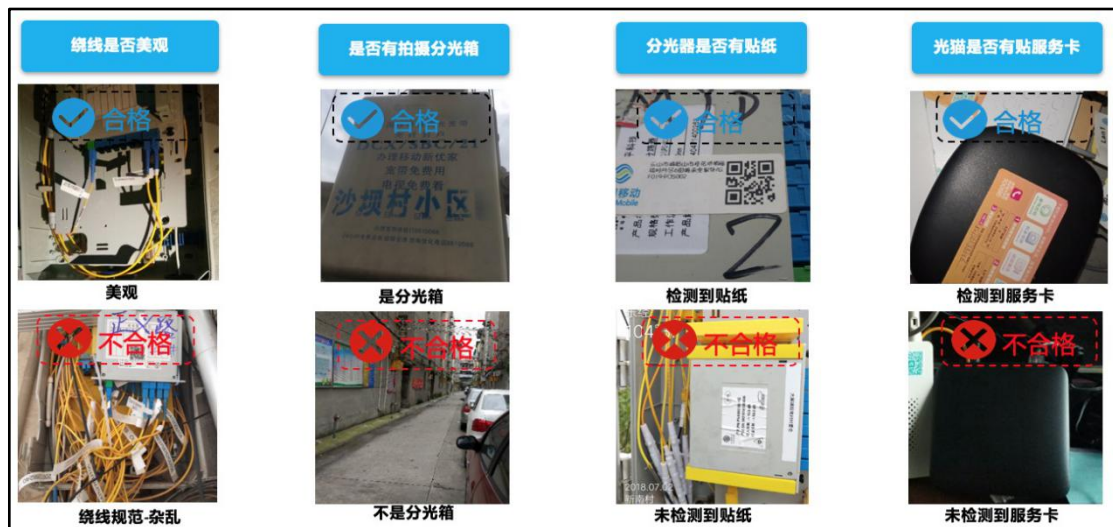
Figure 17: Quality inspection of basic installation techniques
