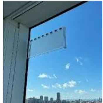
3. Internal CPE antenna provides the best customer self-install option. Smartphone applications can find the best position in the home, usually near a window on the best coverage side of the house. However, there may be aesthetic considerations for the position or location of the CPE.
