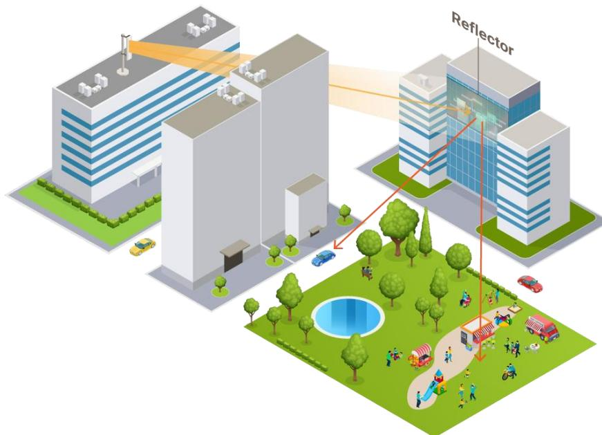
An outdoor NLOS deployment scenario is shown in Figure 13. The signal from the gNB is blocked by tall buildings. By integrating an RIS within the advertising display, the street, park area and walkway could be well covered through the signal redirection. The same deployment scenario could also be applied to stadiums and public squares that are equipped with a large display, and also for office buildings in which a RIS can be integrated into the glass exterior.
