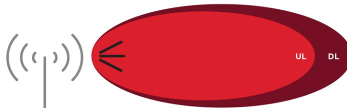
The magnitude of this DL-UL imbalance depends on several factors, including the deployment environment, transmit power of UE and gNB, antenna configurations and antenna gain, among others.
