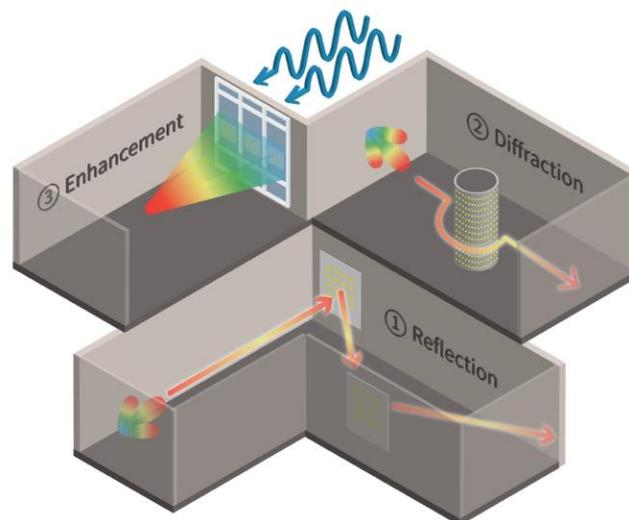
**Reflection** to redirect the signal to expand coverage in a specific area, or create a cold zone elsewhere. This approach is well suited to deployments in office buildings that have installed cubicles and home space. In Figure 15, the reflectors are at an angle to redirect the signal to a specific location, increasing the signal strength by more than 20 dB across office cubicles or multi-room conditions. That would allow the density of small cells to be significantly reduced.
