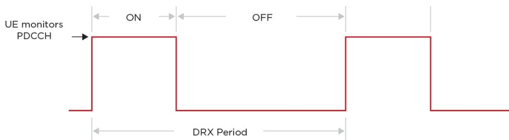
During the ON period, the UE monitors DL signals and channels, such as the Physical Downlink Control CHannel (PDCCH), and performs corresponding data reception. During the OFF period, the UE turns off the transceiver unit and does not monitor DL signals, thereby reducing the UE power consumption. The DRX parameters (e.g., the ON/OFF time period, etc.) can also be dynamically configured to fit different types of services.
