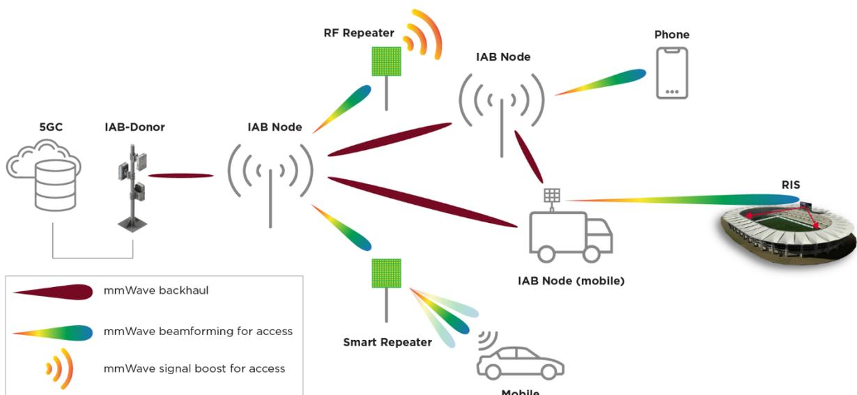
As shown in Figure 8, there are two complementary topologies. A ST (spanning tree) topology enables an IAB node to connect to an IAB-donor via other IAB nodes to support multi-hop connections for backhaul. A DAG (directed acyclic graph) topology creates multi-connections and multi-routes that are used for backhauling redundancy, concurrence for high availability back-up and load balancing purposes.
