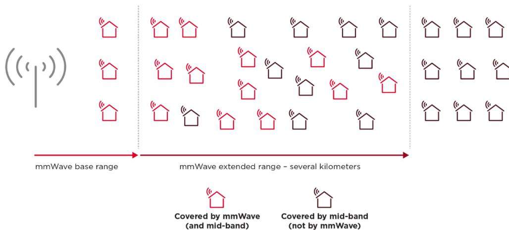
Figure 7 shows a macro-cell site equipped with 5G NR for both mid band and mmWave, in which well-located homes at a range of several kilometres can be served using mmWave extended range.
