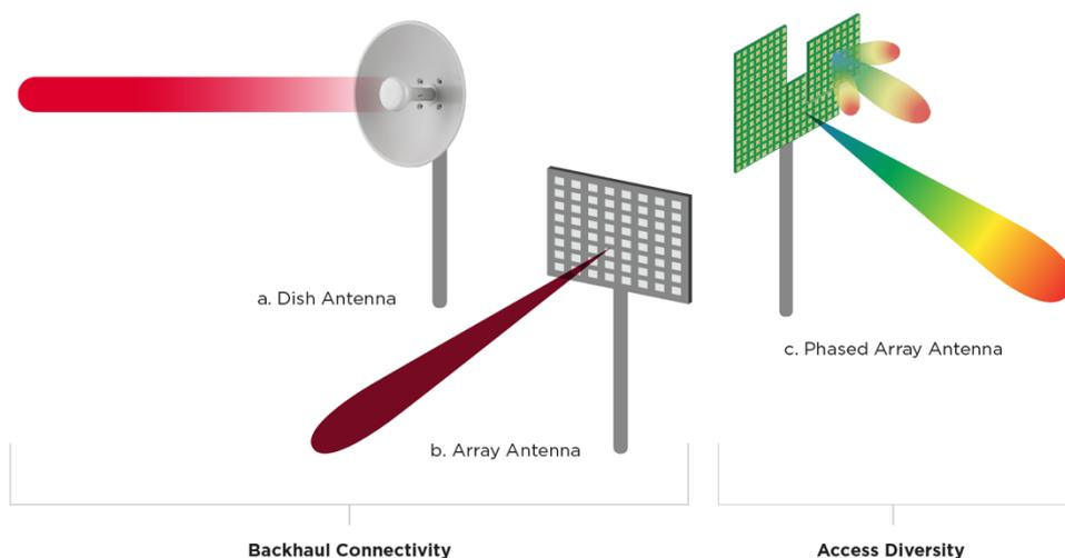
As shown in Figure 10, there are different types of antennas for specific usages. High power and efficient antenna can reduce the number of network nodes required to achieve the required coverage range. As **backhaul connectivity** needs to supply sufficient bandwidth via a static point-to-point connection, high gain and directional antennas that operate in a high frequency band in FR2-2 are well suited to this purpose. The options include:
