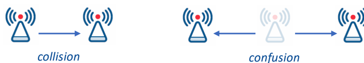
Figure 15 - Collision and confusion conditions between cells of 4.5G or 5G networks
