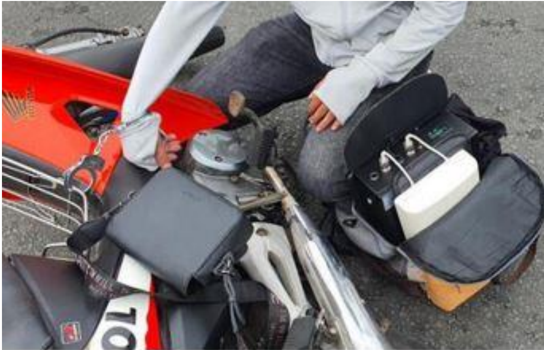
Figure 2 – SMS Blasters are usually placed in a car or in a backpack on a motorcycle driven across different busy areas of a city. (Images from Dan Tri News Agency, dantri.com.vn)
