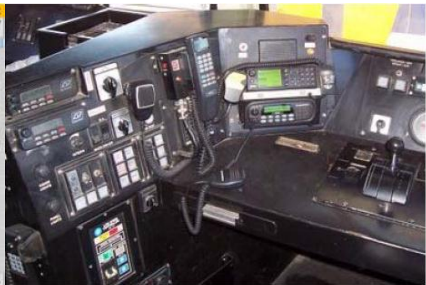
Rationalisation of six separate radio Units per cabin
