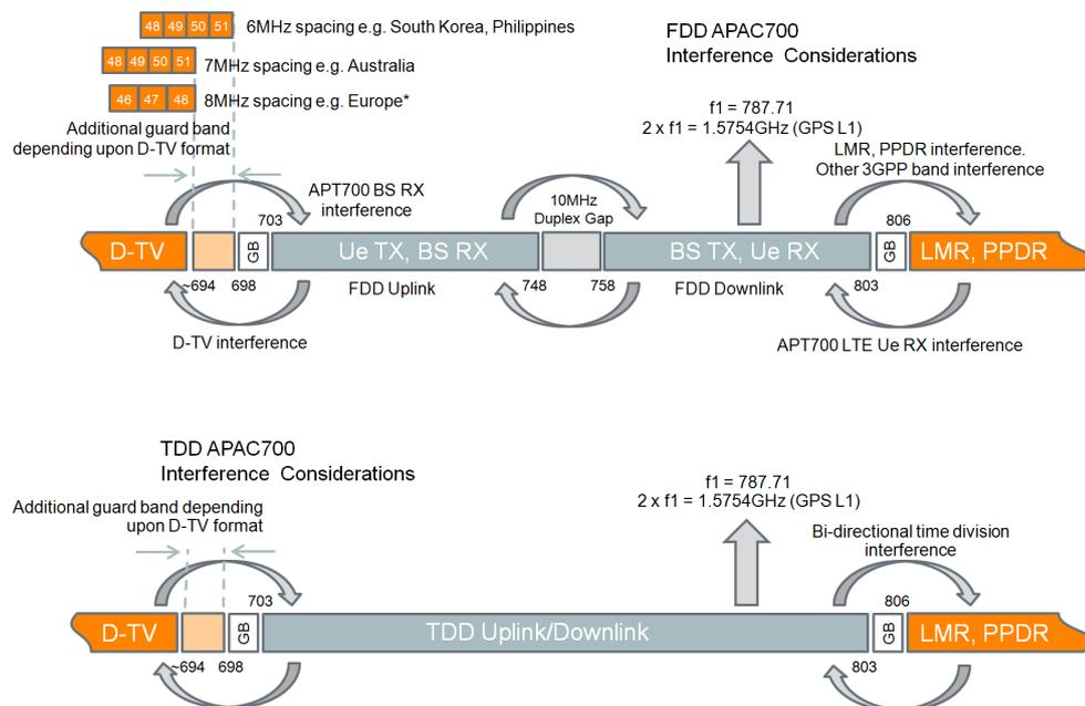
It's also necessary to specifically consider the APT700 TDD case, since with TDD a single channel can be transmitting at one moment in time and potentially causing interference, and the same channel at another moment in time can be receiving and be susceptible to interference.
