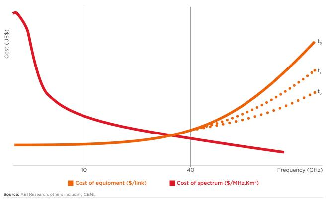
The implementation of novel semiconductor engineering initiatives, such as silicon/germanium chips, has helped push down the cost of equipment curve.
