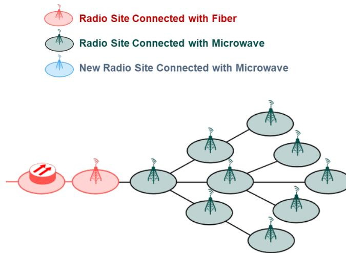
The tree topology of typical networks (as shown in Figure 5) requires distinguishing between tail links (that connect just one terminal mobile site) and aggregation links (which can carry the traffic of multiple terminal sites).
