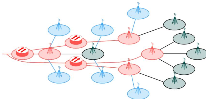
In a star topology (as shown in Figure 6), the increased number of links and more fibre PoPs would allow for a more efficient network densification.
