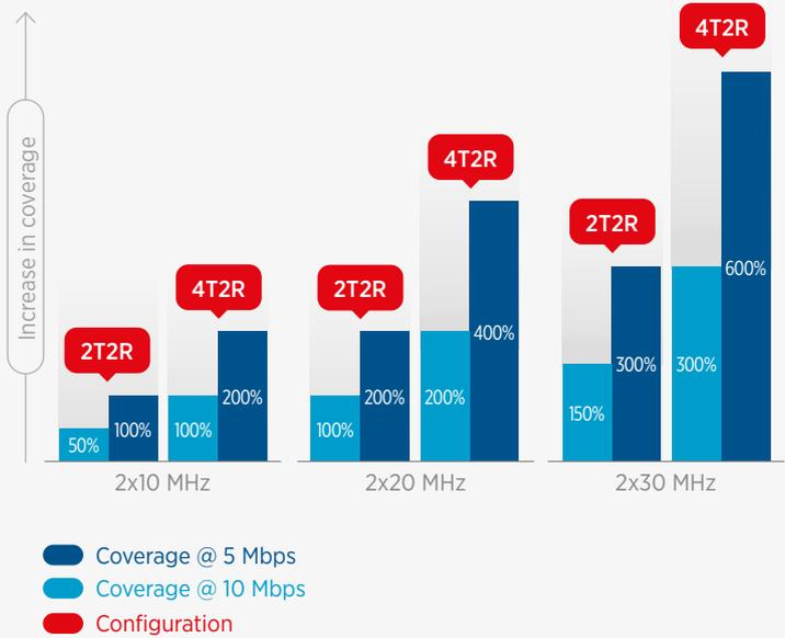
Impact of bandwidth and MIMO configuration on cell-edge speed coverage compared to a base (100%) of 2x10 MHz with a 2T2R configuration with a 5 Mbit/s speed target.
