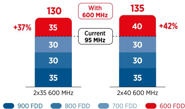
The first scenario for Region 1 shows the potential downlink speed increase for 2x35 and 2x40 additional 600 MHz spectrum without the use of the 20 MHz of SDL spectrum in the 700 MHz band.
