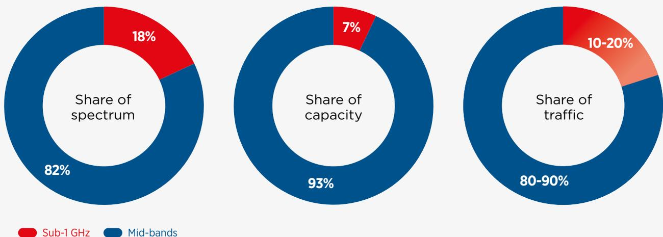
Low-band spectrum is limited. Comparing the MHz volume of spectrum with mid-band, low band typically accounts for around 18% of spectrum and mid-bands for 82%, depending on the country. This calculation includes spectrum on spectrum assignment roadmaps that is not yet assigned to mobile operators.
