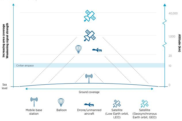
AERIAL NETWORKS - WIDER AREA COVERAGE, WEAKER SIGNAL, LOWER CAPACITY (SOURCE: GSMA INTELLIGENCE)
